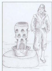
Figure 4. The huayra was the most sophisticated smelting furnace developed in the Andes. It operated by catching the wind through perforations in its body. In the illustration, a huayra with its operator, according to a record made at the end of the 19 th century, in Bolivia.
