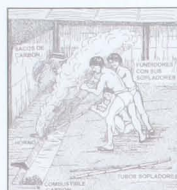
Figure 3. In Batán Grande, northern Peru, copper-arsenic bronze was produced on a large scale. The smelters used small furnaces dug in the ground and blow pipes to attain the necessary high temperatures (redrawn by SHIMADA & MERKEL 1991).
